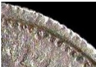
Rim damage left by edging post strike
