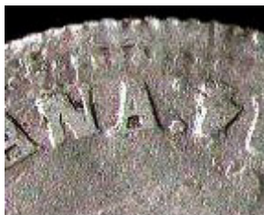
Rim damage left by edging post strike
