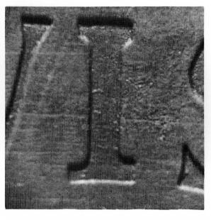
8&9: The letter-punch which was used to punch both of the "R\*s" into the original dies had a flaw in the form of a small notch which shows clearly on the outside of the top curved portion.
