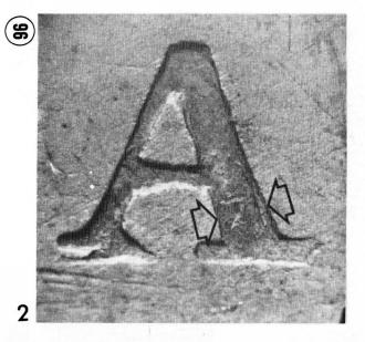
The process that was used to duplicate the original managed to reproduce many of the smaller details but failed when copying the heavy portions of most the lettering since they show considerable reduction in thickness.
