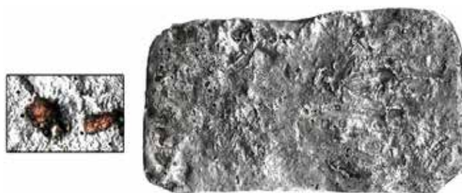
Embedded chunks of pure copper in "tumbaga" bar # M-83
