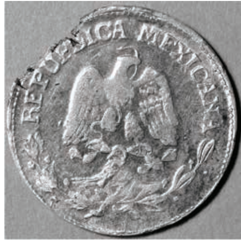
Plate 3. C.M.G.R.O. 1915 50-centavos GB-162-VAR, dies (5/A). This is a 10.87g silver strike, with the planchet punched out near the edge or end of strip (note the planchet flaw). A specific gravity of 10.13 was obtained from this piece, suggesting a silver planchet of approximately 0.77 fine, likely a peso planchet of semi-refined silver bullion.
